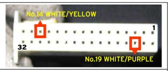
Using a generic connector pin estractor, gently draw out the No.14 terminal (white/yellow wire) and No.19 terminal (white/purple wire) from the 32 pin black connector and swap the two terminals.
